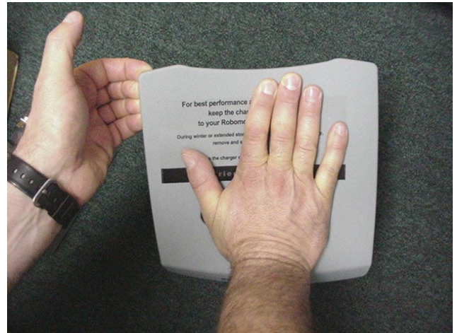
Picture: Removing the power pack cover by pulling up at its corners, one corner at a time
