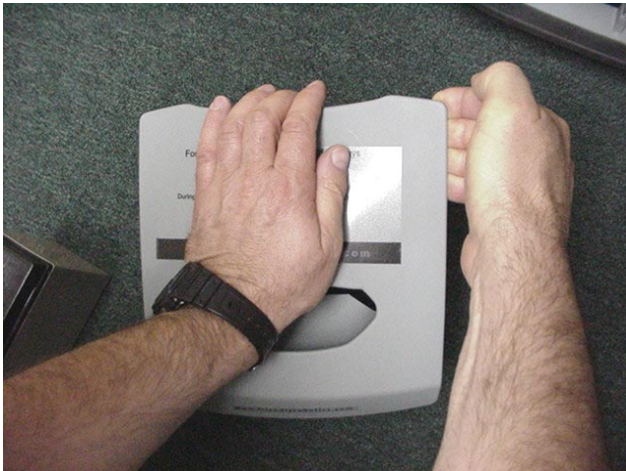
Picture: Removing the power pack cover by pulling up at its corners, one corner at a time
