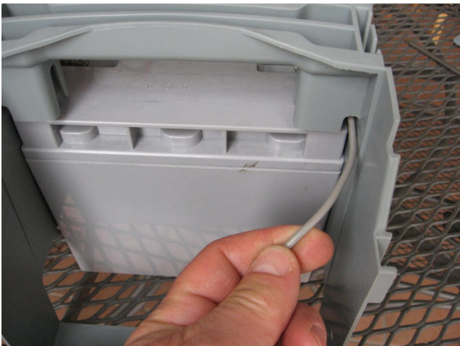
Picture: Power pack case placed on top of front battery and then Grey wire pulled backwards through small opening under the power pack case handle – shown bellow as well
