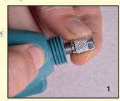
4. Attach the correct sharpening stone by slowly turning chuck while simultaneously pressing lock button until it engages. (FIG 2)
