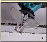
4. When all the teeth on the top of the bar have been sharpened, use a glove or rag to advance the chain by pulling towards the end of the bar. Sharpen remaining cutters evenly.
